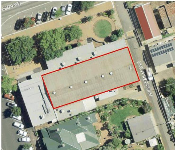
Figure 3: Asbestos roof to be removed and replaced
