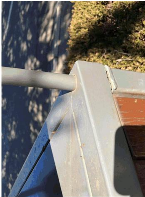
Bin: Cracked metal frame (Vinnies)
