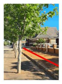
Underground root barrier installed along footpath nature strip to prevent surface roots causing any future property damage
