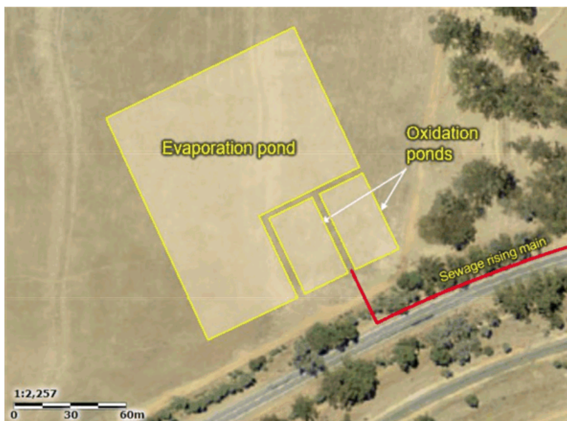
Figure 4-4: Springdale treatment sub-option A – proposed STP layout
