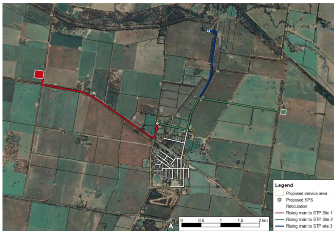
Figure 3-2: Proposed reticulation layout and transfer options for Ariah Park
