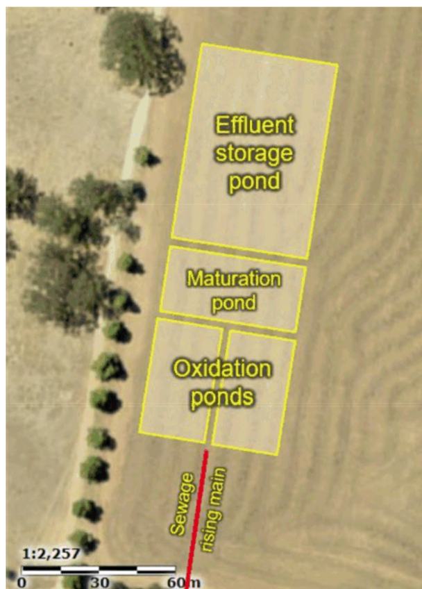
Figure 4-6: Springdale treatment sub-option B – proposed STP layout
