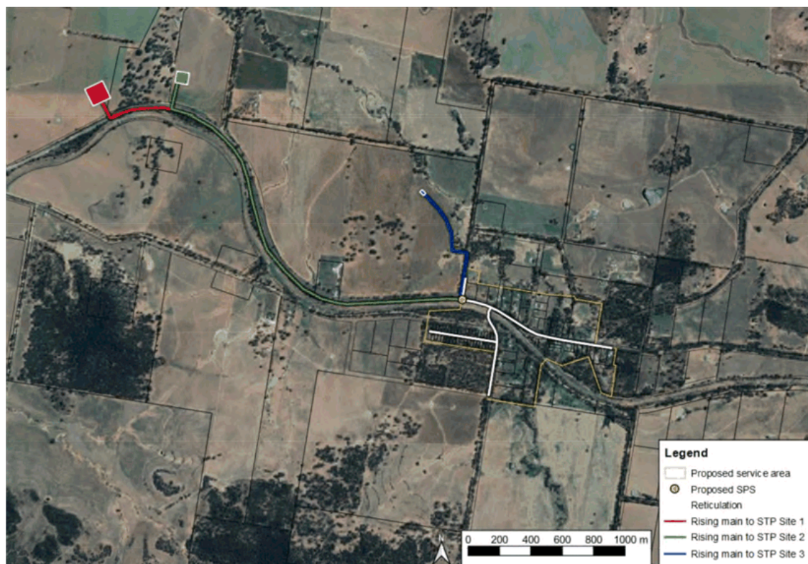
Figure 4-2: Proposed reticulation layout and transfer options for Springdale
