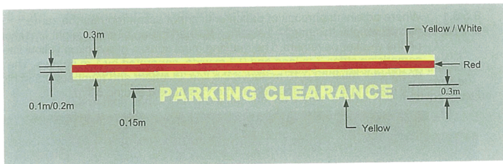
Figure 8.5-1: Parking clearance line
