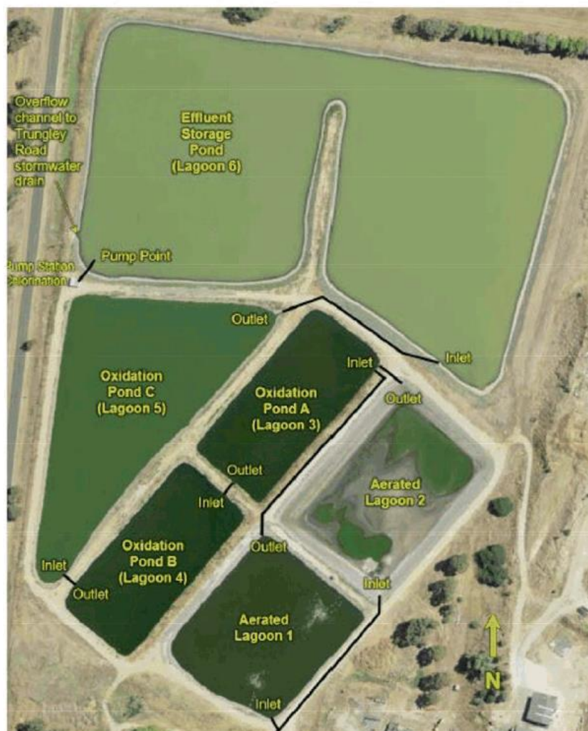
Figure 5-3 – Layout of the Temora STP
