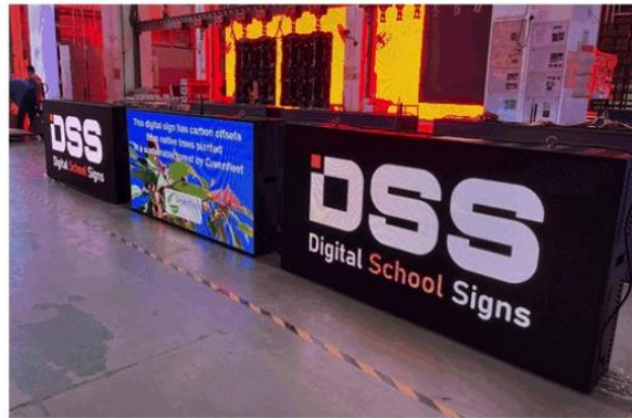
Digital School Sign LED screens being age tested at the Ledman factory.
